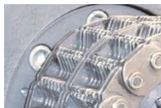
Drive chain with reinforcement plates, combination of center and side guide
