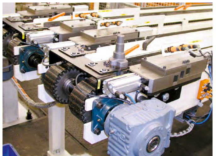
Heavy duty multi-lane storage systems for cast iron or forged parts
