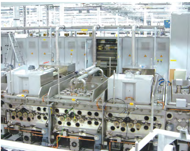
Biflex inverted tooth chains in vacuum coating equipment for solar cells
