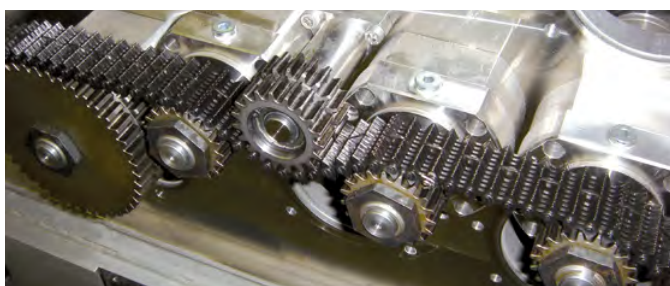
Biflex inverted tooth chains. Roller drives with specially coated inverted tooth chains for use in vacuum applications
